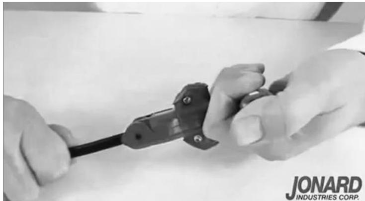
**Figure 5 – Pull the cable splitter along the cable to slit the jacket.**
