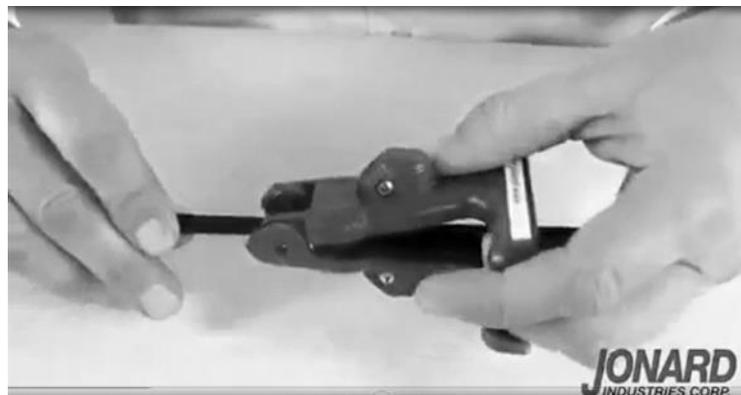
**Figure 4 – Position the cable slitter over the cable and close the tool.**
