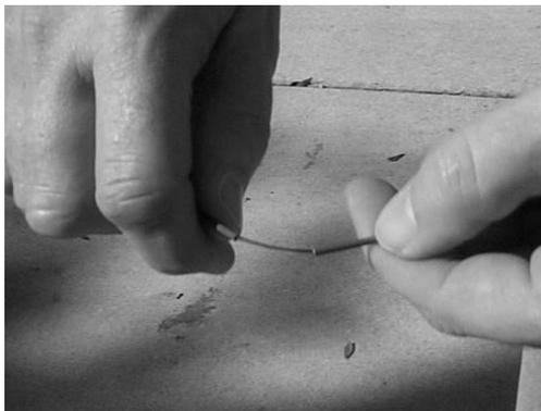
**Figure 9 – Flex and snap the buffer tube at the score line.**
